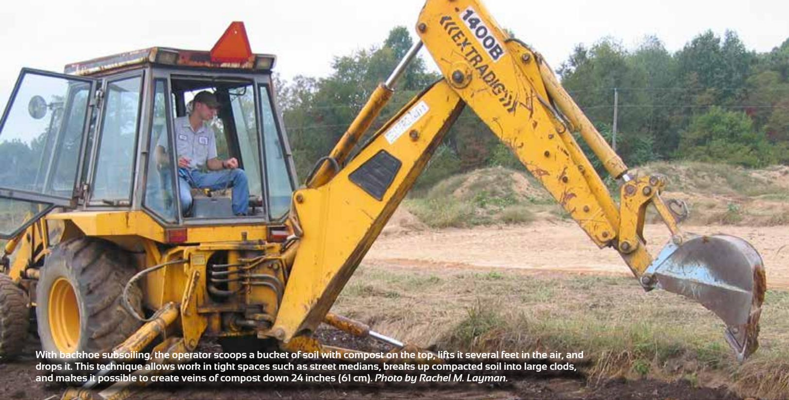
With backhoe subsoling, the operator scoops a bucket of soil with compost on the top, lifts it several feet in the air, and drops it. This technique allows work in tight spaces such as street medians, breaks up compacted soil into large clods, and makes it possible to create veins of compost down 24 inches (61 cm). Photo by Rachel M. Layman.
