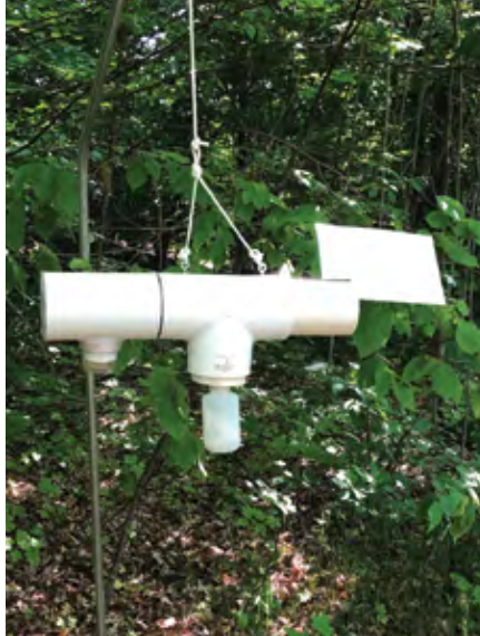
Figure 3: Beetles were collected from 2018 to 2020 using wind-vane traps baited with bread dough bait and pheromones.
